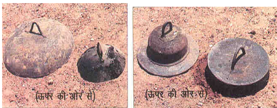
Figure 10: The photo on left is of uninsulated coal feedhole covers used in BTKs; the photo on the right shows the improved insulated feedhole covers
