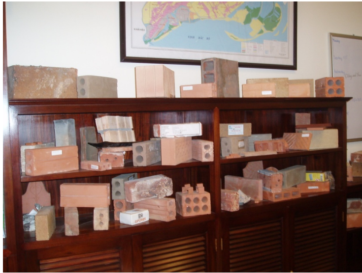
Figure 20 A variety of perforated and hollow bricks produced in Vietnam
