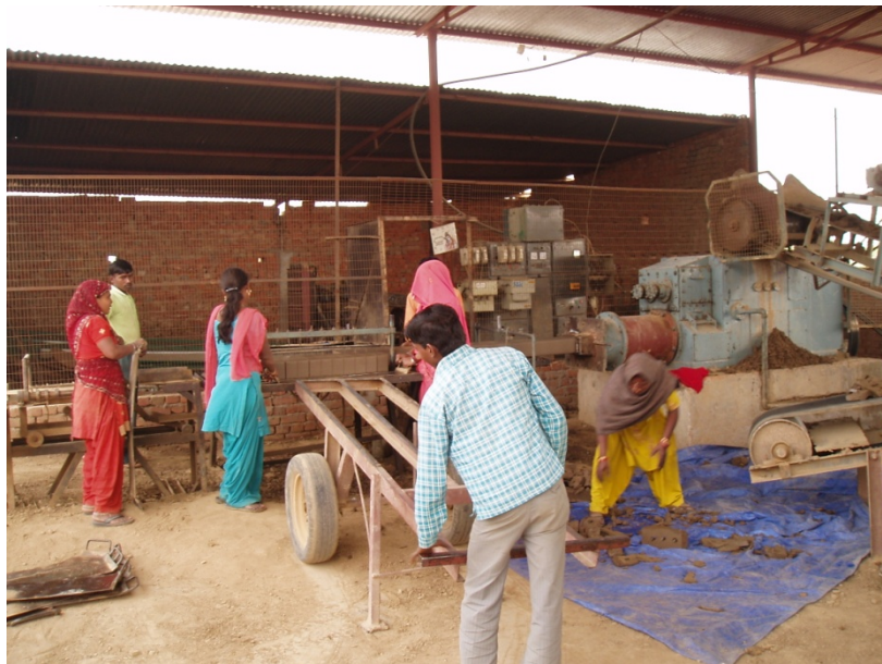
Figure21 An extruder for making perforated bricks near Chandigarh (India)
