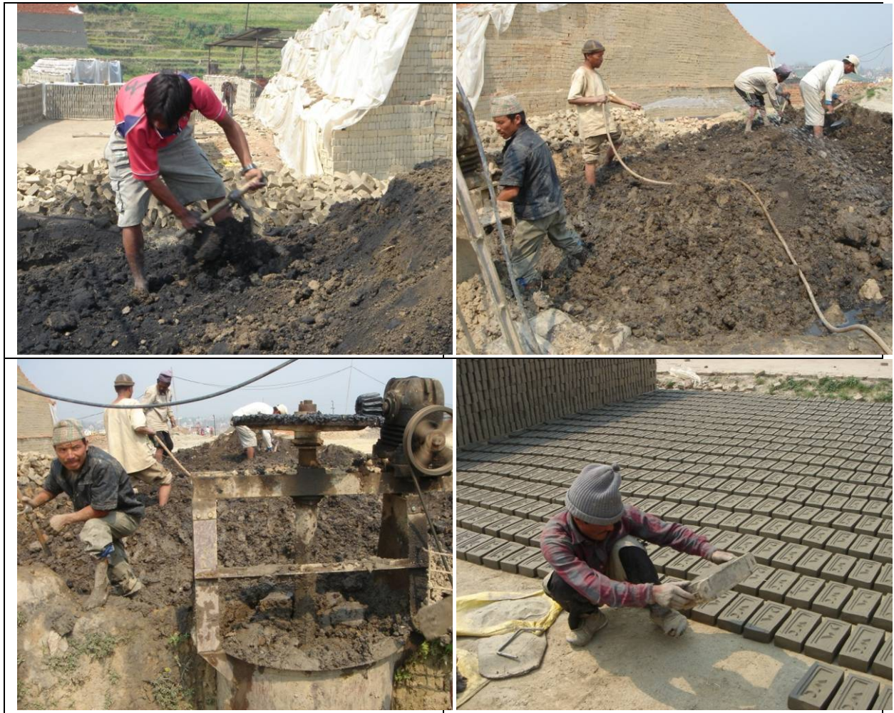
Figure 18. Manual addition of internal fuel followed by mixing in a mechanized pug-mill 21
