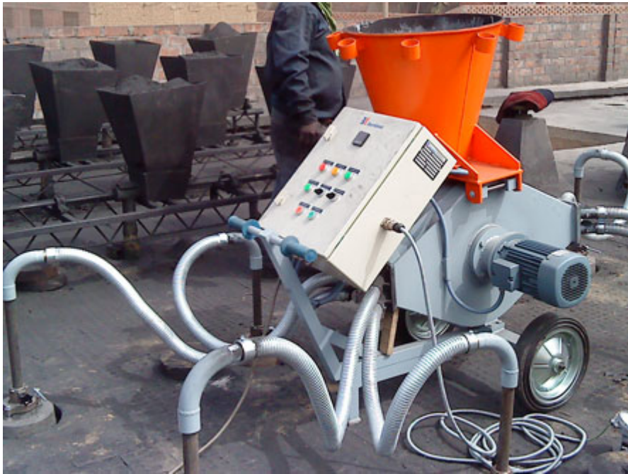
Figure 19. Solid fuel burners having a fuel crushing and distribution unit
