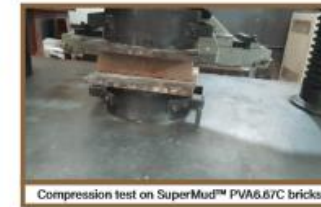
Compression test on SuperMud™ PVA6.67C bricks
