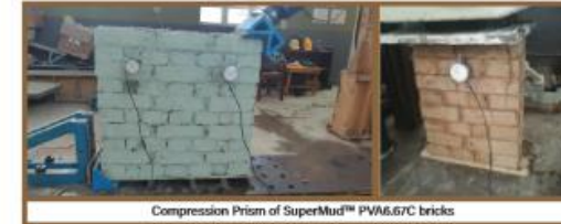
Compression Prism of SuperMud™ PVA6.67C bricks
