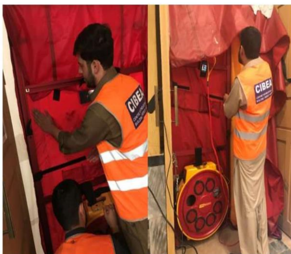
Team CIBEA setting the blowerdoor equipment
