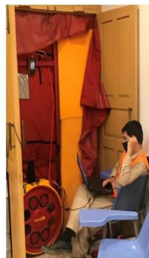
Taking depressurization readings
