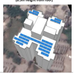
Non-Elevated Structure Configuration (0.5m height from roof)
