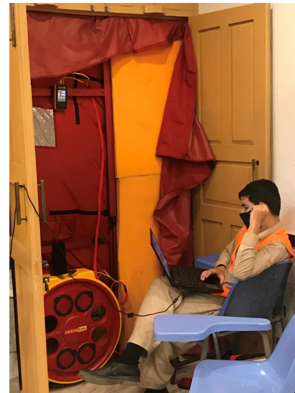
Taking depressurization readings
