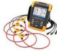
1. Energy Analyzer (KW, KVA, PF, Harmonics)
