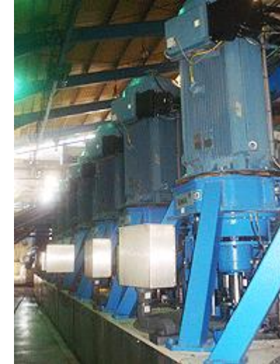
Sugar centrifuges fitted with ABB Motor and VFD at Al Khaleej sugar mills centrifuges
