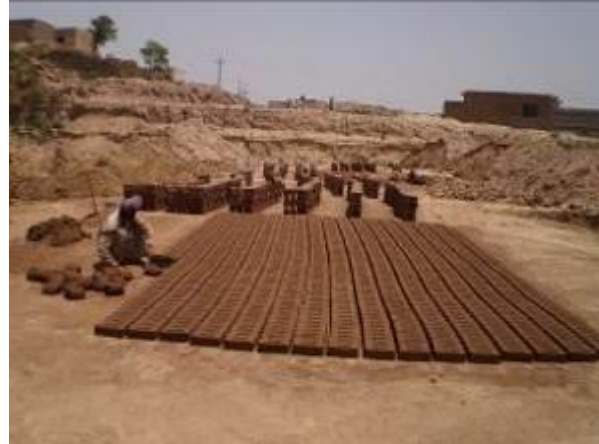
Photos: Manual moulding of bricks using steel moulds
