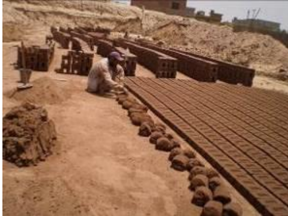
Photos: Manual moulding of bricks using steel moulds
