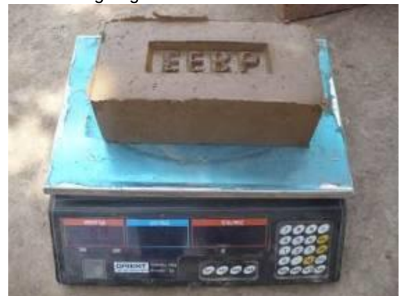
Photo : Weighing bricks for moisture contents
