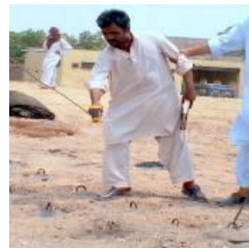
Photo:.. Temp gun recording stoking holes
