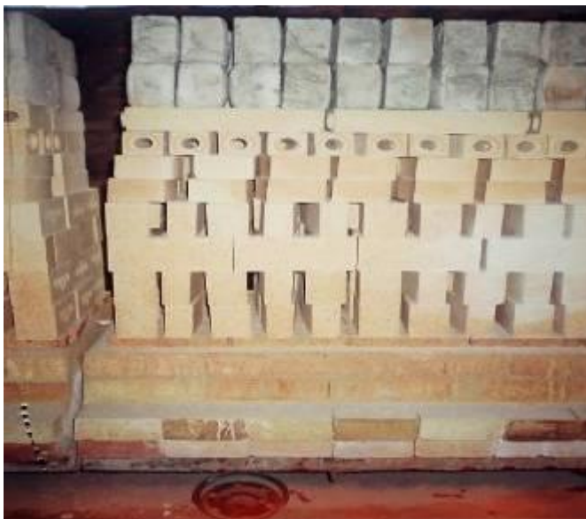
Photo: Bricks loaded on a fire wagon
