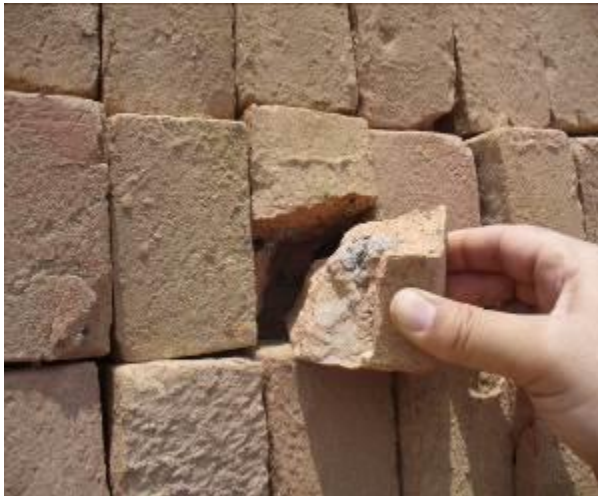
Photos: Anomalies like pebbles burst open the bricks
