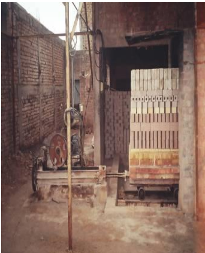
Photo: Bricks loaded on a fire wagon
