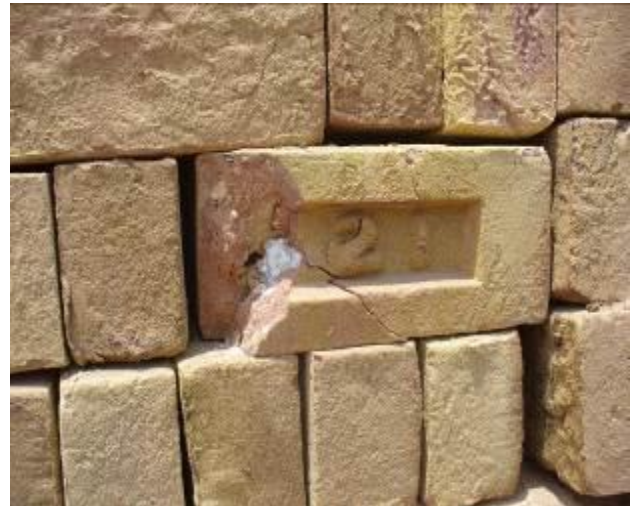
Photos: Anomalies like pebbles burst open the bricks
