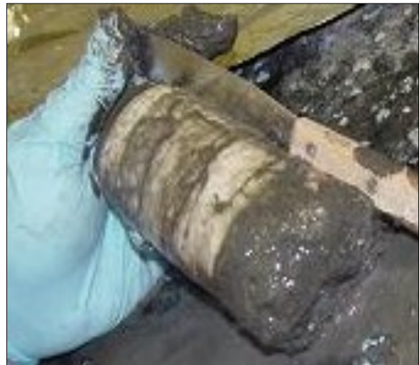
Figure18: Gas hydrates in fractured shales in Deep water area of K-G basin, India
